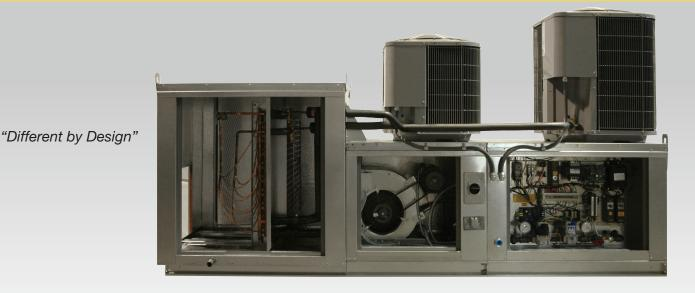
The Modular Packaged Unit by Grease Master is a factory packaged air conditioning and heating unit for 100% Outdoor Air (OA) applications. Units are ideal for tempering makeup air and are sized to operate between 360 to 600 CFM/ton of cooling.
